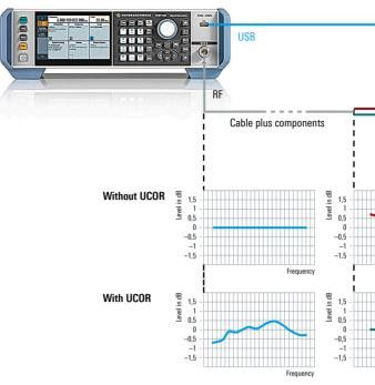
correction values are automatically determined and saved in the UCOR table. When UCOR is activated, a frequency response compensated RF signal is available at the new reference plane for the DUT.
