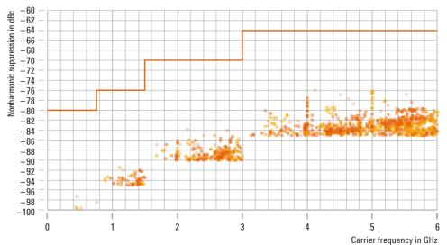
When testing ADCs, for example, excessively high nonharmonic components in the analog signal can lead to problems. The R&S®SMB100B excels with very low nonharmonic signal components of < -76 dBc (specified) at 1 GHz. Measurements show significantly better results.
