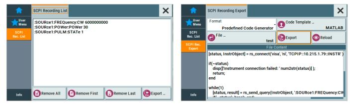
The built-in SCPI macro recorder and code generator supports fast, easy generation of SCPI program sequences.
